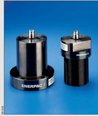
Enerpac work supports provide either additional non-fixed location points to the clamps, or support to larger or thin section workpiece components, always in order to minimize workpiece deflection during machining. The Collet-Lok® design does not require hydraulic system pressure to maintain support position.
