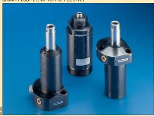
Hydraulic pull cylinders utilize hydraulic pressure to hold down parts in a fixture. The guided plunger maintains orientation during the full clamping cycle, eliminating the need for an external guide. Internally threaded plunger ends accept various custom attachments to assist in the clamping process.
